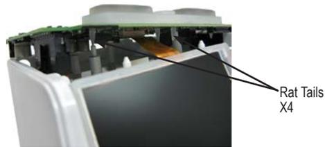
10. Align the LCD display ribbon connector with the PC board's connector and push into place without damaging the ribbon.
