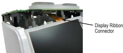
5. Lift PC board out of the main chassis until the main wire harness connector is accessible.
