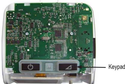
9. Position the keypad so that the Ramp key is on the front right of the new PC Board. Pull the "rat tails" through the corresponding holes in the new board using needle nose pliers. Ensure that the "rat tails" are pulled completely through the board with the keypad flush with the top of the board.
